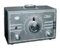
The model 200 is a resistance capacitance type for making frequency response, distortion and other audio measurements. Ranges: 30-300, 300-3,000, 3,000-30,000 cps. Output: 10 v into 500 ohm load. Less than 1% rms harmonics 30-15,000 cps with 500 ohm load. Response: Better than  $\pm 1$  db 30-15,000 cps. Calibration Accuracy: 3% of scale reading. Size:  $13\frac{3}{4}$ " x  $7\frac{1}{4}$ " x  $9\frac{1}{2}$ ". For operation from 105-125 v ac 50/60 cps. Shipping Weight: 17 lbs.
